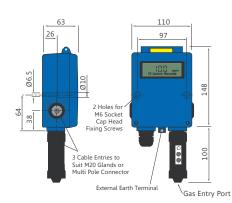
2 Holes for M6 Socket Cap Head Screws Fixing Screws External Earth Terminal 2000 (standard)
