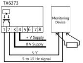
A pull up resistor may be required at the monitoring device.
