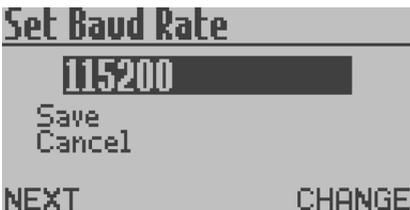
Press **R** to navigate to the required **Baud Rate**, press **L** and select **Save** or **Cancel** as required. Press **R** to confirm the selection and return to the **Output Setup Menu**.
