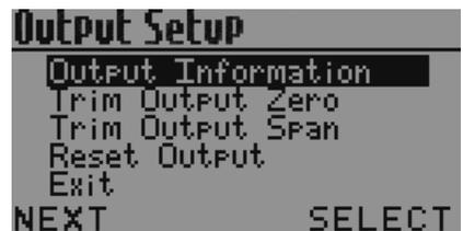
Press **L** to navigate to **Increase** or **Decrease** as required. Press **R** to **Increase** or **Decrease** the **Output Zero** as required.
