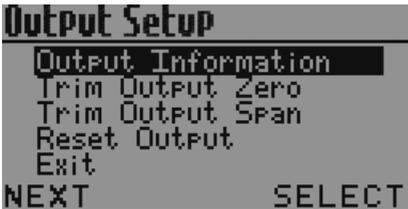
From the **Output Setup Menu** press **L**, navigate to **Trim Output Span** and press **R** to enter the **Trim Output Span Menu**.
