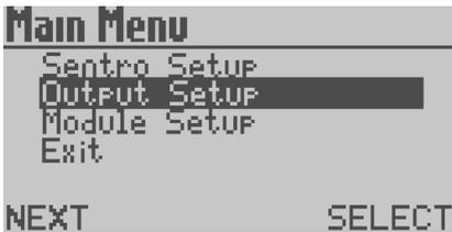
From the **Main Menu** press **L**, navigate to **Output Setup** and press **R** to enter the **Output Setup Menu**.
