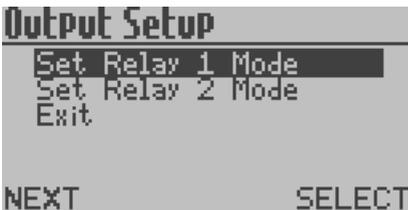
From the **Output Setup Menu** press **L**, navigate to **Set Relay 1 Mode** or **Set Relay 2 Mode** and press **R** to enter **Set Relay 1 Mode** or **Set Relay 2 Mode**.
