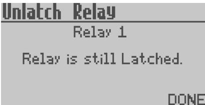
Press **L** to navigate to **Unlatch Relay 1** or **Unlatch Relay 2** and press **R** to confirm the selection.
