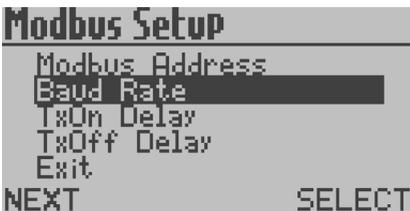
From the **Output Setup Menu** press **L**, navigate to **Baud Rate** and press **R** to enter the **Set Baud Rate Menu**.
