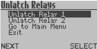
From the **Unlatch Relays Menu** press **L**, navigate to **Unlatch Relay 1** or **Unlatch Relay 2** and press **R**.
