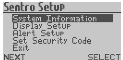
From the **Sentro Setup Menu** press **L**, navigate to the **System Information** and press **R** to display the **System Information**.
