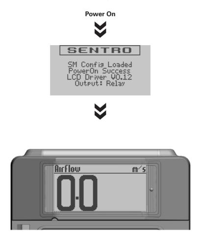
After five seconds the **Main Display** will appear. The **Main Display** displays the current airflow.
