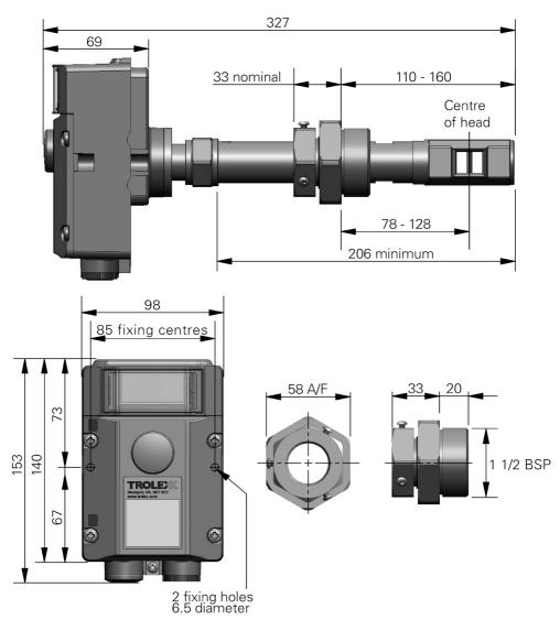
All dimensions in mm Probes available from 160 to 2000 mm insertion length in 100 mm increments
