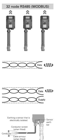
communicate with the master unit on a single data cable.
