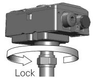
Rotate the sensing probe or the sensor housing to the desired position.
