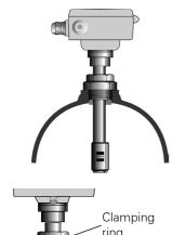
Clamping ring 1/3 diameter Fit a corresponding threaded boss or flange at the monitoring point and install the sensor, ensuring a gas tight seal.
